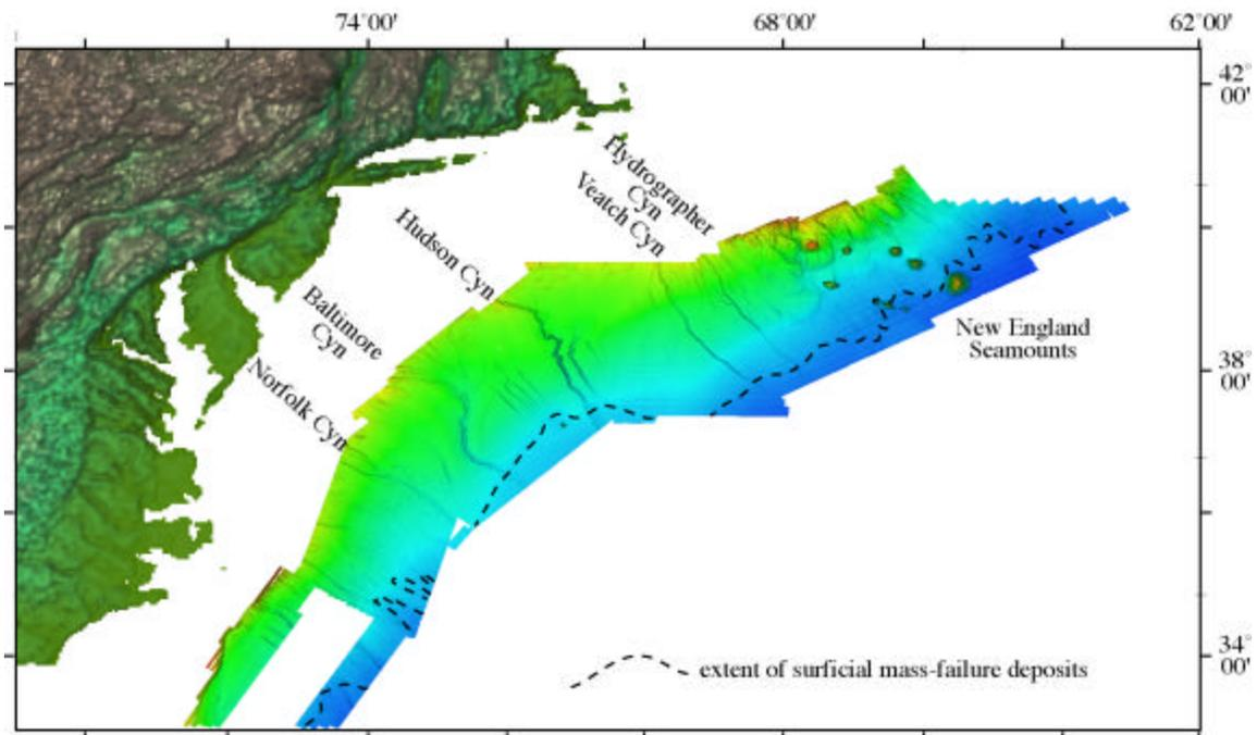
Figure 7. Multibeam color-coded bathymetry of the US Atlantic continental rise. Only a few of the submarine canyons have been labeled. Dashed line shows approximate extent of surficial mass-failure deposits.
