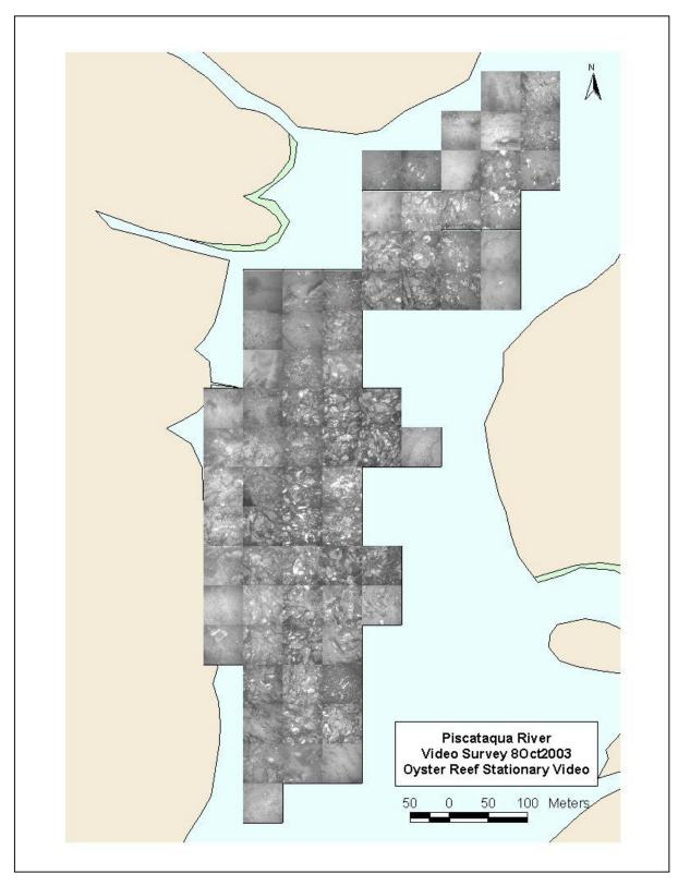
Figure 8. Piscataqua River reef photomontage based on stationary video imagery. Each individual photo is about  $0.5 \times 0.5$  m, and each corresponds to one of the stationary video sites shown in Figure 2.
