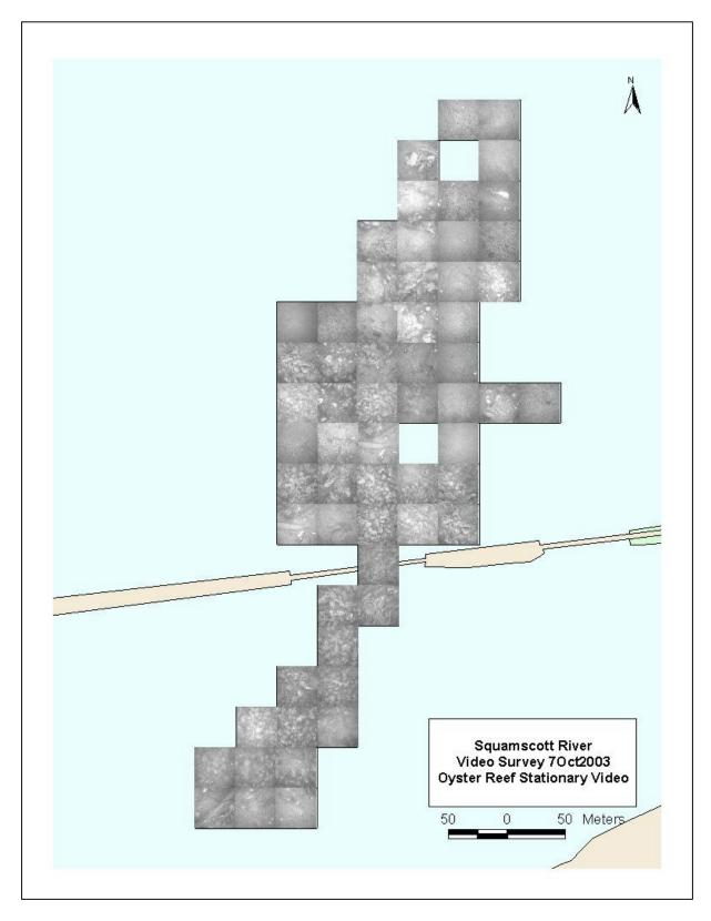
Figure 9. Squamscott River reef photomontage based on stationary video imagery. Each individual photo is about  $0.5 \times 0.5$  m, and each corresponds to one of the stationary video sites shown in Figure 3.
