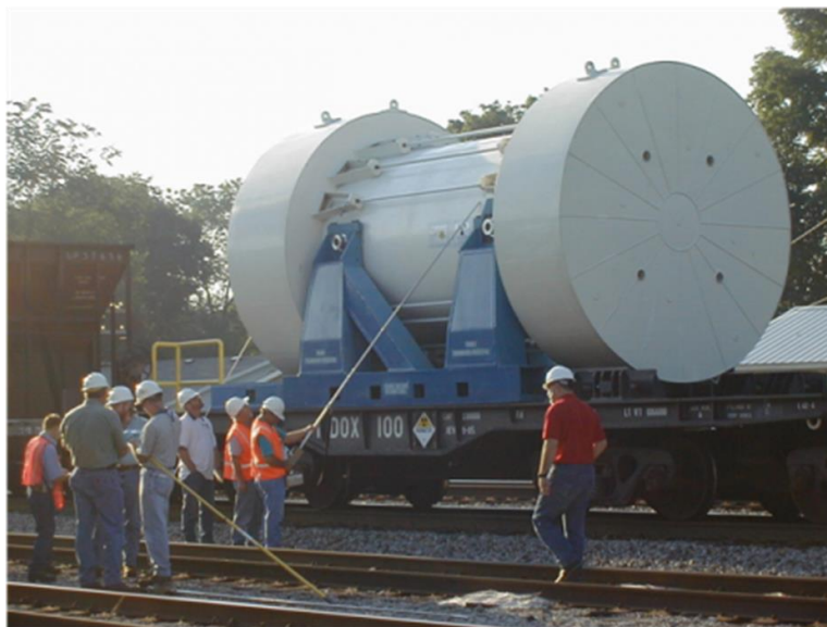
Figure 1: Spent nuclear fuel rail transportation cask (U.S. Department of Energy)
