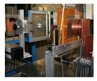
Fig. 4. Sample frame at PIF, showing irradiated samples and control samples (at bottom).
