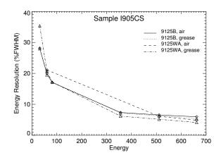
Fig. 1. Energy resolution as a function of energy for a Saint-Gobain sample of LaBr<sub>3</sub>. The resolution depends slightly on the optical coupling and on the type of glass in the PMT.
