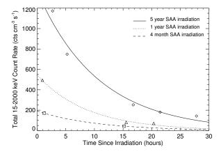
Fig. 14. Total internal counting rate (15-2000 keV) due to activation in LaBr<sub>3</sub> for three different proton fluences.
