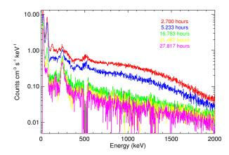
Fig. 10. Internal background due to activation in the 5-year-irradiated Saint-Gobain LaBr<sub>3</sub> sample at various times after irradiation.
