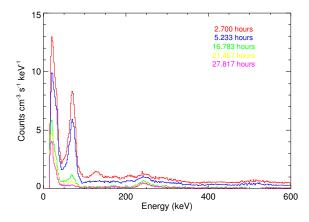
Fig. 11. Internal background lines below  $600\ keV$  due to activation in the 5-year-irradiated Saint-Gobain LaBr $_3$  sample.
