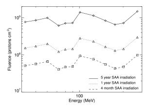
Fig. 3. Proton fluence spectra generated at PIF. The samples were exposed in three batches to represent the total fluence expected from the SAA after 4 months, 1 year, and 5 years in orbit. Note that the bin size increases at higher energies.
