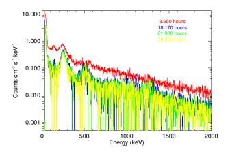
Fig. 12. Internal background due to activation in the 5-year-irradiated Saint-Gobain LaCl<sub>3</sub> sample at various times after irradiation.
