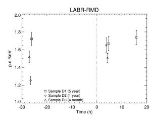
Fig. 6. Photoelectron yield of Saint-Gobain LaBr<sub>3</sub> sample exposed to 5-year SAA irradiation. Control sample is also plotted.
