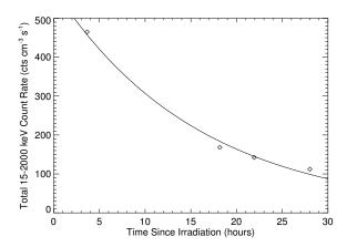
Fig. 15. Total internal counting rate (15-2000 keV) due to activation in LaCl<sub>3</sub> for a proton fluence equivalent to 5 years of SAA passages.
