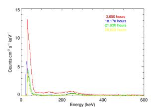
Fig. 13. Internal background lines below 600~keV due to activation in the 5-year-irradiated Saint-Gobain LaCl $_3$  sample.
