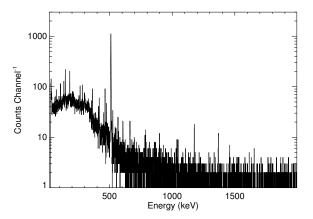
Fig. 9. Ge spectrum of activation lines from Saint-Gobain LaCl<sub>3</sub>, 1.3 hours after irradiation with 5-year SAA proton fluence.
