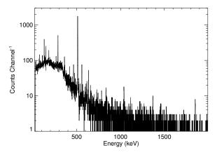
Fig. 8. Ge spectrum of activation lines from Saint-Gobain LaBr<sub>3</sub>, 1.2 hours after irradiation with 5-year SAA proton fluence.
