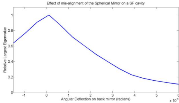
Figure 16a: Mis-Alignment of the back reflector: A slight mis-alignment can reduce the light through the system; a deflection of about 10^{-4} radians would cause a 20% loss through the system. For comparison, an angular deflection on this order would correspond to a shift of 1mm over 10 meters. This is doable with the experimental system.
