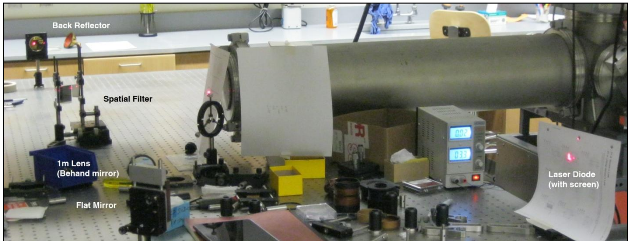
Figure 9: The Full optical system. Here, all components are visible, as explained in the other sections. The laser diode has a piece of paper in front with a small hole (1cm by 1cm) cut in it. This is so it becomes easy to view the back-feedback coming through the system. Also seen is the two angular control knobs for the flat mirror, which are used as the proxy for aiming the laser diode.
