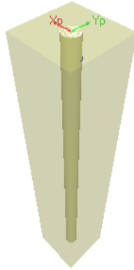
Figure 4: Cylinder Pile Model
