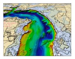
For example, some maritime tasks may be better suited to a blended chart and multibeam shaded relief model of bathymetry. Other tasks might decimate the chart to just a safe water contour, the shoreline, and the key buoys.
