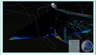
GeoZui4D can be used to reconstruct data from multiple sources. Here are shown EK60, DeltaT and the reconstructed whale track from DTAG. The cross section of three whales can clearly be seen in the Imagenex Delta T multibeam data.
