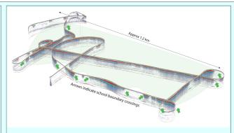
On July 27th, 2009 the boundaries of a school of prey were delineated by steering the RV Auk in and out of the boundary. The Auk is a NOAA research vessel operated by the Stellwagen Bank National Marine Sanctuary. It was equipped with an Simrad EK60 single beam fisheries research sonar with a 38kHz transducer and a 120kHz transducer.
