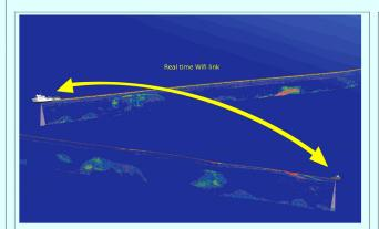
Researchers on either ship can see all data in an interactive 3D environment updated in real time. The ships were linked via a wireless network which carried real time sonar data allowing an integrated immediate display of the current situation in GeoZui4D.
