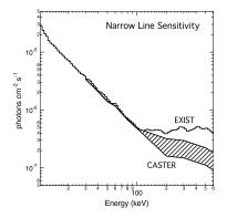
**FIGURE 2.** The estimated narrow line sensitivity for CASTER as compared to published sensitivity of EXIST ( $5\sigma$  sensitivity, one-year exposure). The hatched area represents a range of possible sensitivity values for CASTER depending on the assumptions for the background scaling.
