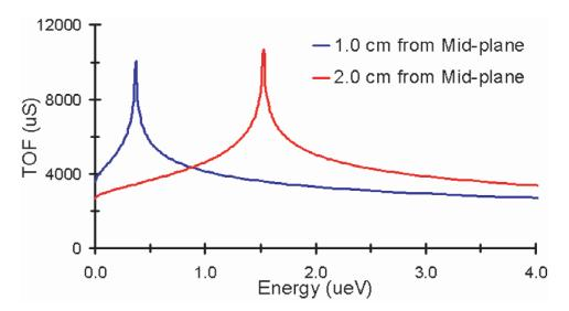
Fig. 3. TOF plots for a simulated proton with energy  $0 \mu eV$  to  $4.0 \mu eV$  created on the central axis of the spectrometer. Initially, the proton is traveling in the direction of increasing potential and has velocity in the direction of the central axis.
