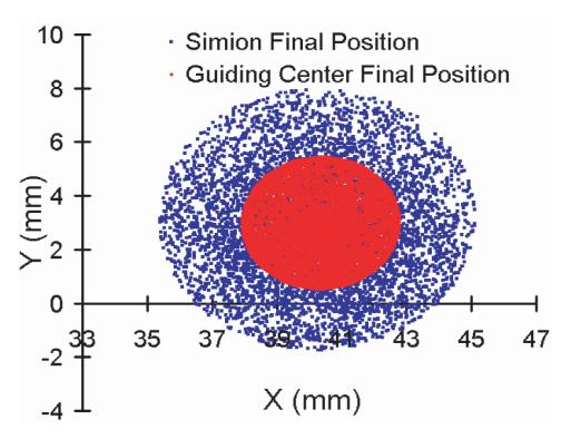
Fig. 7. Proton final positions generated by SIMION compared to proton guiding center final positions generated by the custom software.
