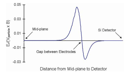
Fig. 4.  $E_r/(V_{\text{particle }}B)$  vs distance for a simulated off-axis proton. The trajectory of the proton goes through  $E_r$  maximum.
