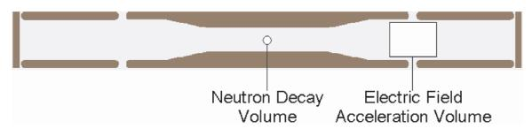
Fig. 2. 2D schematic of the abBA spectrometer showing location of the neutron decay volume and the electric field acceleration volume.
