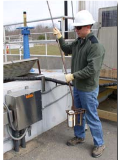
In 2008 PREP staff sampled effluent from eight wastewater treatment facilities in the Great Bay Estuary watershed to determine the nitrogen input into the system.
