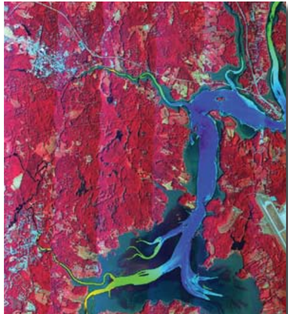
Hyperspectral aerial images record 64 wavelengths across the visible and near-infrared spectrum. The resulting imagery was used to map water clarity, macroalgae, and eelgrass in the Great Bay Estuary.
