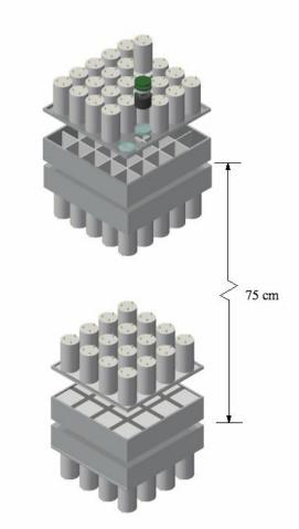
**Figure 4**. A 10 cm  $\times$  10 cm subsection of the model Compton telescope using deuterated liquid scintillator for D1 and LaBr<sub>3</sub> for D2. See text for details.
