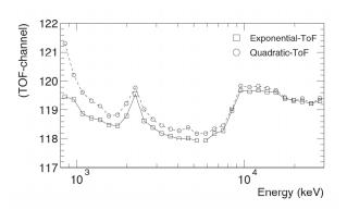
**Figure 2**: Centroid of the COMPEL ToF peak as a function of energy.
