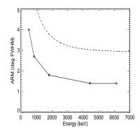
Figure 6: Angular resolution of the scintillator Compton telescope as measured by the ARM. Dotted line indicates values for COMPTEL.
