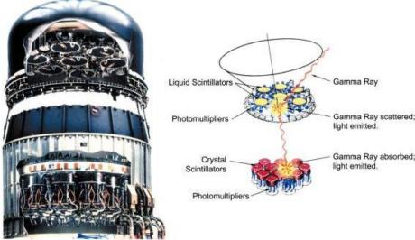
**Figure 1**. A photo montage of the COMPTEL instrument and a graphic illustrating the method of detection, where  $\gamma$  rays scatter in the upper detector assembly (D1) and are absorbed in the lower (calorimeter) detector assembly (D2) with the resulting restriction on the incident photon direction.
