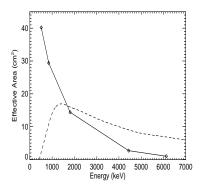
Figure 7: Effective area of the example scintillator Compton telescope for the data cuts given in the text. Dotted line indicates values for COMPTEL.
