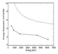
**Figure 5**: Energy resolution (%FWHM) of the LaBr<sub>3</sub> scintillator Compton telescope vs. energy. Dotted line indicates values for COMPTEL.
