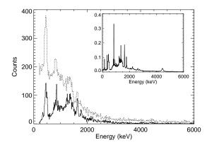
Figure 10: Simulated solar flare spectrum (inset) as measured by the  $LaBr_3$  Compton telescope (solid) and monolithic NaI detector (dotted).
