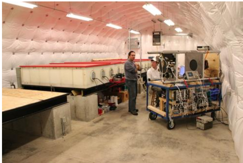
Fig. 6. Field measurement before the installation of \sim 10^3 kg of lead in a neutron monitor.
