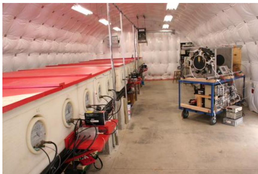
Fig. 7. Field measurement after the installation of the lead in a neutron monitor.
