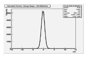
Fig. 5. A measured 0.7 cm position resolution in a rod.
