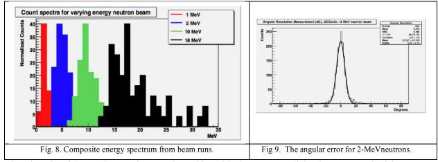
In Fig. 9 is a plot of the angular error between the position of the beam target and the closest approach of the event cone. The distribution is narrow with a  $\sigma_{\Theta}$  of 5.2° at 2 MeV and 4.8° at 10 MeV. Even though the signal strength is much greater at 10 MeV, the angular resolution is driven by the geometrical uncertainties in the locations of the scatters and the small size of the instrument.
