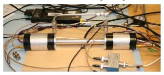
Fig. 3 A rod liquid scintillator detector.
