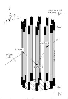
Fig. 2. A fully populated radially symmetric neutron imager.
