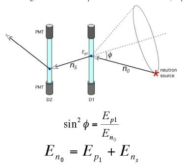
Fig. 1. Schematic of a double neutron scatter in two cylindrical organic scintillator detectors.
