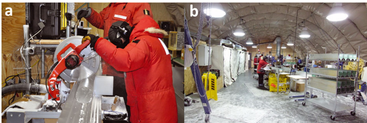
Fig. 6. (a) View of the 'Cutting' station and the dry-cut circular saw used to cut the runs of ice core into 1 m long sections. (b) View of the inside of the core-handling arch. A roller rack full of 1 m long sections of ice core is on the right. The person in the middle of the photo is at the 'Electrical properties' station. The white rectangular booths on the left of the photo are the drying booths.
