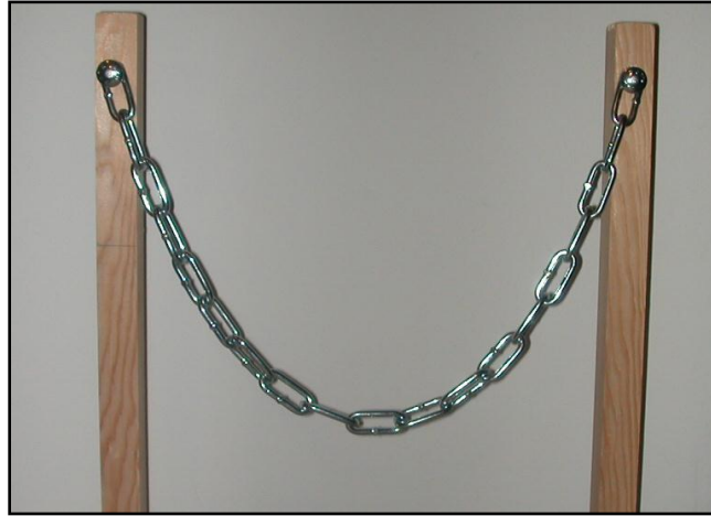
Figure 30: Hanging chain forming a catenary shape
