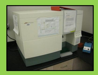
Flow Cytometry: Each solution sample is run through a flow cytometer. This machine uses laser scattering to detect the size, granularity, and fluorescence of individual cells. These properties are directly proportional to the amount of light that is scattered.
