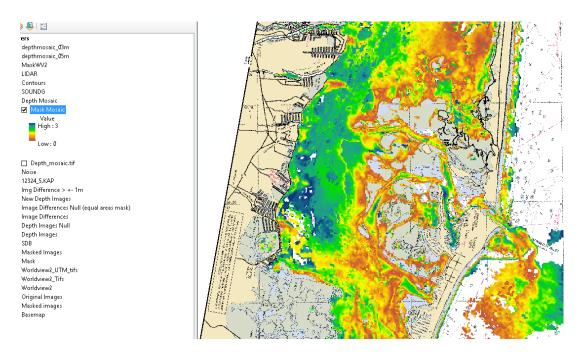
**Figure 3.** Mosaic produced from stable depth areas – based on subsequent image pair comparisons.
