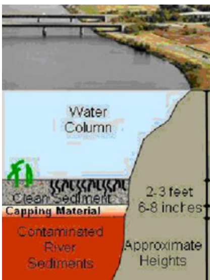
An example of reactive capping of river sediments
